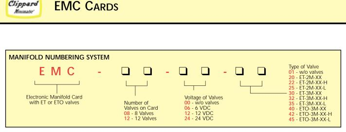
EMC-08-00-01 and EMC-12-00-01 are part numbers for cards without any valves, and without manifold. Manifold mounting hardware is included. Manifolds may be ordered separately, if desired.
